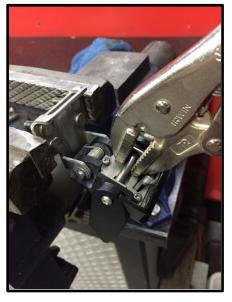
4)Remove the vise-grip, now remove the shaft, install the Rickter-RRP hook, install the shaft and tighten the screw. It is recommended to use Loctite on the screw.
