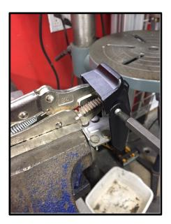
2)Put the latch assembly in a vise and using vise-grips pliers hold the shaft so you can remove the Philips screw
