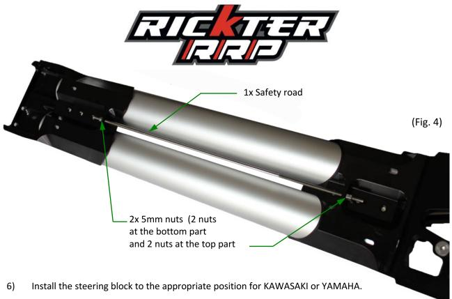
The KAWASAKI owner will have to do a bit of filing to fit the cable. The block is designed to fit both but requires some filing to fit the KAWASAKI. Install the cable in the slot and use the washer included in the kit to block the cable.
